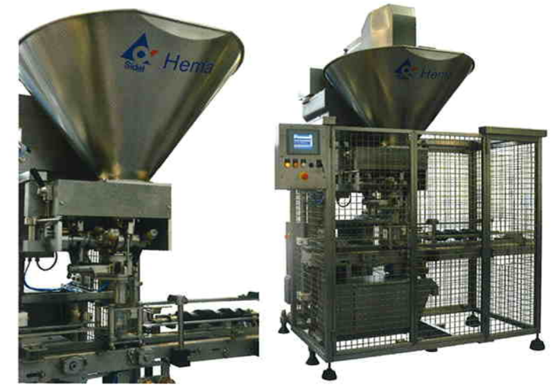
The operator console on the HEMA MV filler is equipped with a touch screen.
